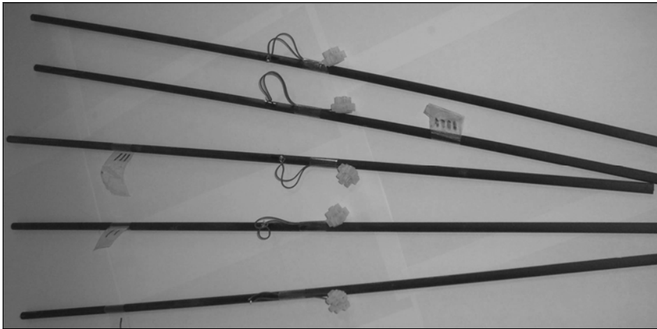
Figure 5.26 The five rods used during the tests with attached strain gauges and connectors
