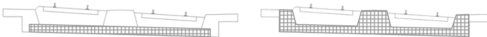
Figure 7.33 Area of the bridge’s cross section involved in bearing capacity calculations. Left: Original area; Right: New area
