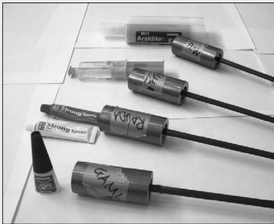
Figure 5.18 The four types of glue tested and assembled 85 mm anchorages from the fifth design
