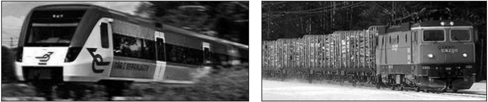
Figure 7.22 Left: Regina train with controlled and constant axis weight; Right: Freight train with randomly distributed and varying axis weight
