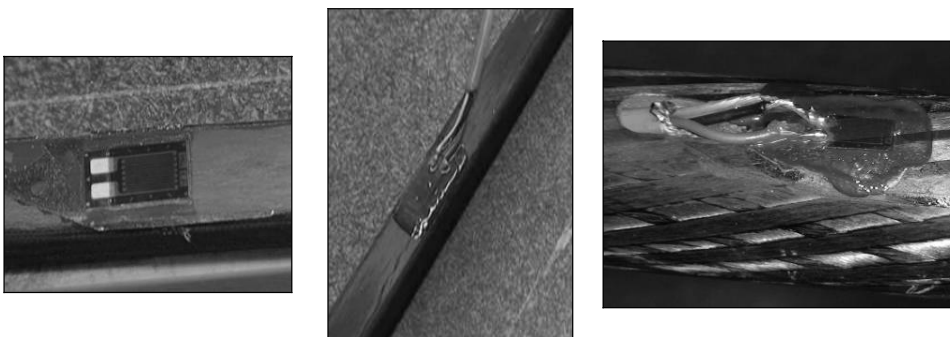
Figure 7.19 Left: Strain sensor glued to an NSMR bar; Centre: Strain sensor on NSMR with protective coating and soldered cables; Right: Strain sensor on tube, protected and with cables connected
