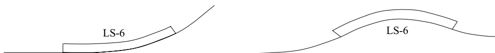
Figure 6.11 Compression of LS-6 in front of the wedges back end and tension of LS-6 when the back end of the wedge is at the longitudinal position of the sensor
