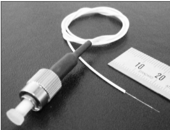
Figure 5.29 Optical fibre where the fibre can be seen as the outermost 4 mm in the right part of the picture. Also the two protective layers and a connector are seen
