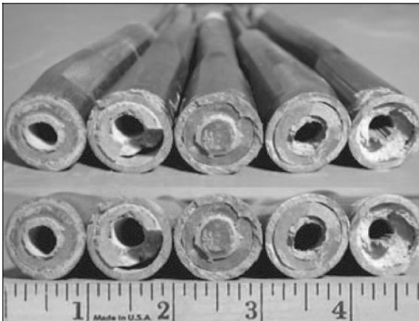
Figure 2.25 Steel sleeves held by hydraulic grips after pull-out of CFRP rod, Koller et al. (2007)
